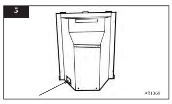
5.5 Gas pipe entry must come through the right-hand side of the box. The rubber seal must be cut using a sharp knife to allow the isolating elbow to pass through it. Ensure the rubber is not damaged when doing this.
